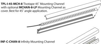
**INF-C-CHAN-8** Infinity Mounting Channe with lens for LED protection in tight spaces.
